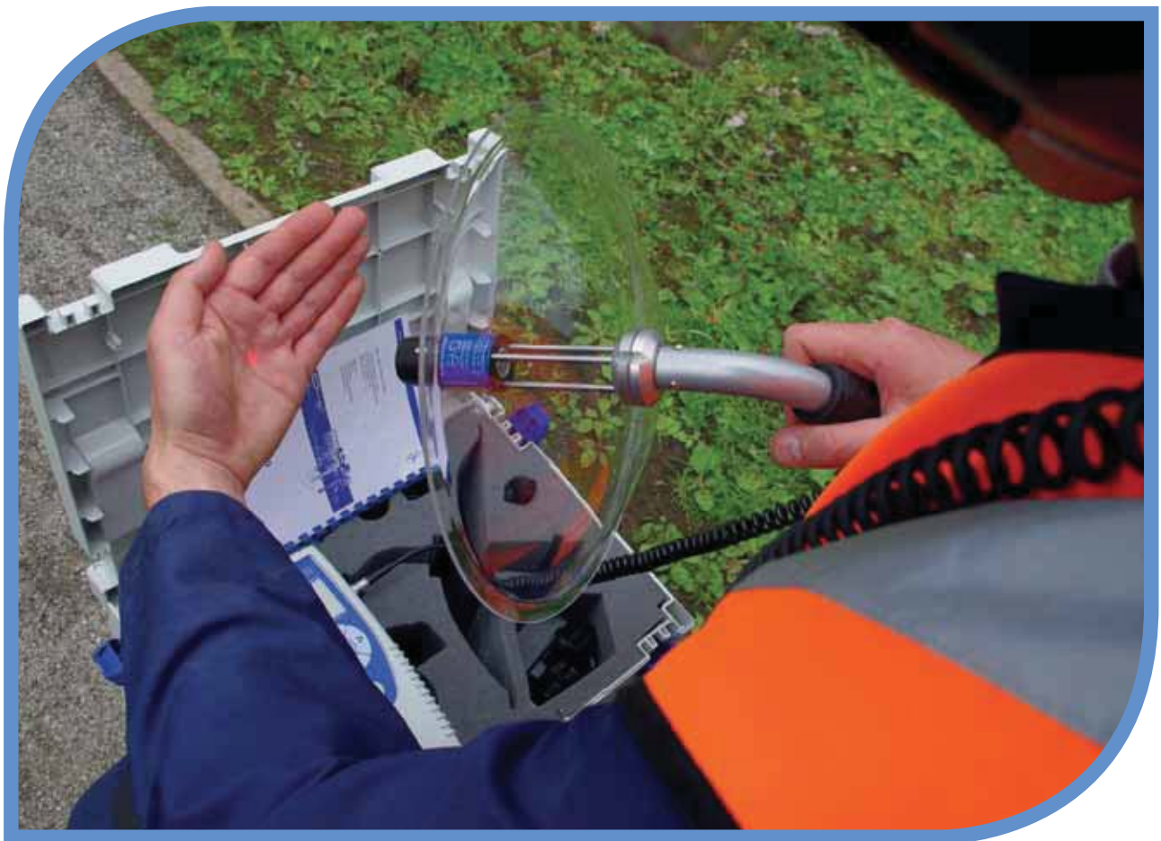
The UltraDish™ has a precision laser sight built in.
