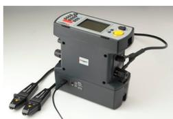
The DLRO10 and DLRO10X may be also powered from an optional mains / line power supply unit the DLRO10LPU. This unit is simply fitted to the instrument in place of the standard battery pack.
